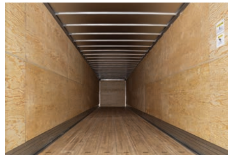
Standard wood lining with exterior grade plywood.
