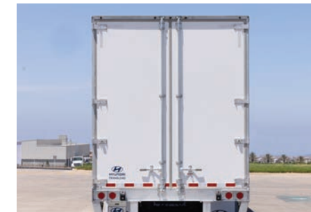
Rear frame has 0.19" thick hot-dipped galvanized steel construction with low profile header, tube shaped posts.
