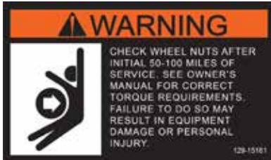
Warning for wheel nuts inspection
